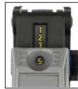
Stepped Stripping Depth For Reduce Friction
